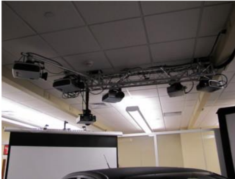
Figure 3.2 – Projectors responsible for producing the driving environment [42].
