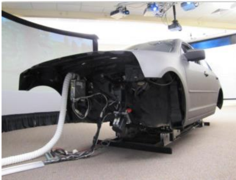
Figure 3.3 – Ford Fusion mounted on one-degree-of-freedom motion platform [42].
