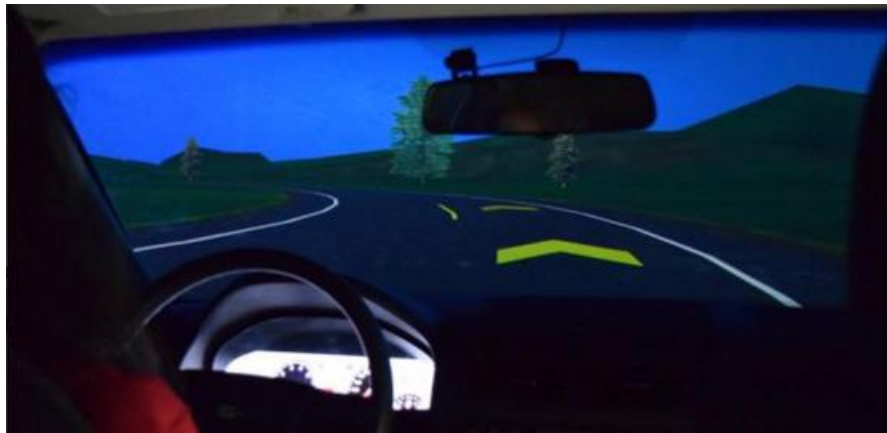
Figure 3.8 – Example of the holographic projection chevron alignment warnings.
