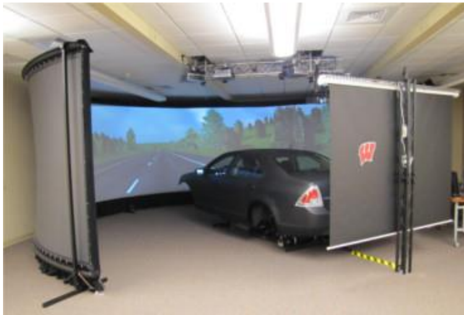
Figure 3.1 – UW – Madison TOPS lab driving simulator [42].
