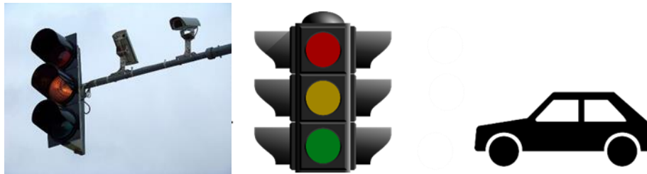
Figure 3.1 – Detection systems at a signalized intersection
