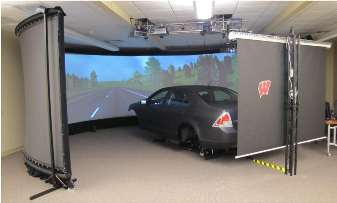
Figure 4.1 – Full-scale driving simulator at UW-Madison
