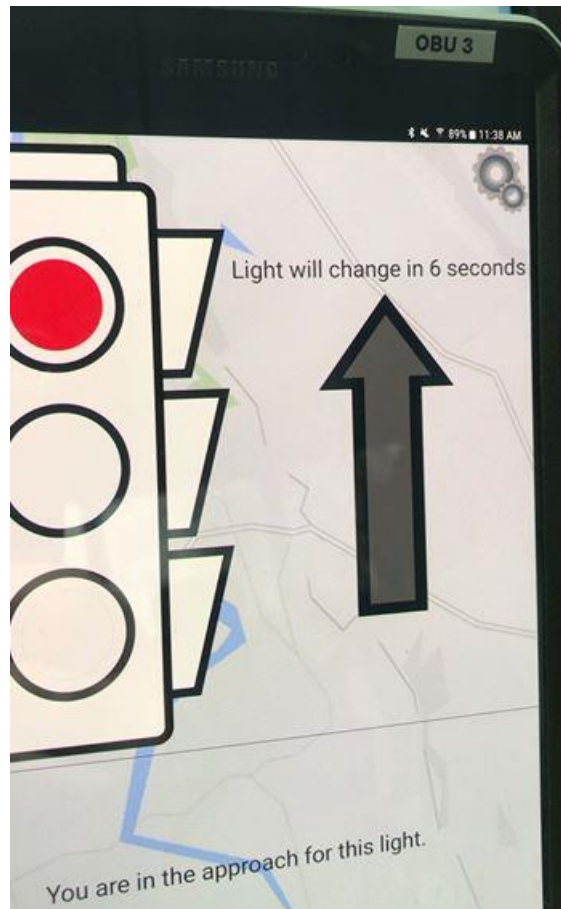
Figure 3.4 – SPaT interface showing signal phase and progression
