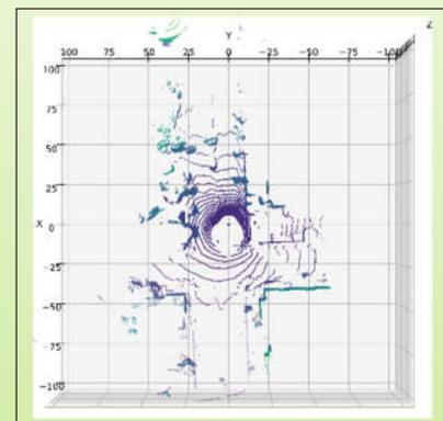
Bird-eye view of simulated lidar data.
