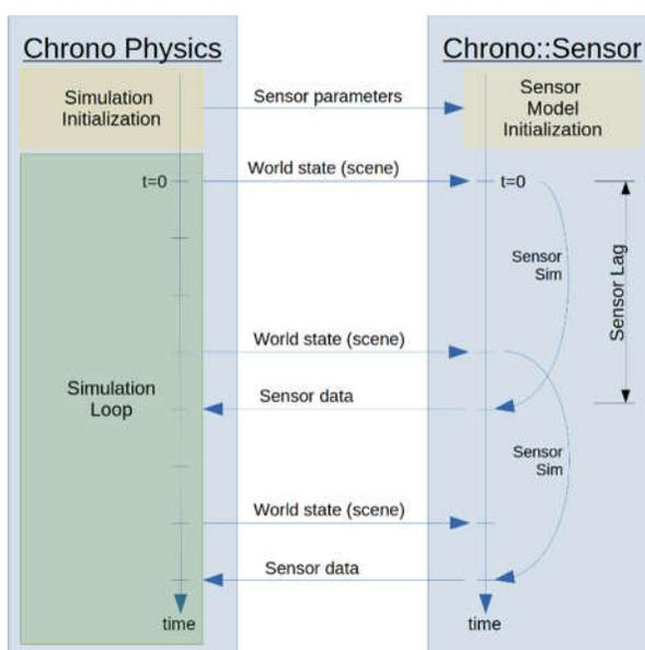
An illustration of the connection between Chrono and Chrono::Sensor shows the ability for dynamics to control the evolution of the environment. Data is generated with parameterized lag, update frequency, and sensor-specific models, and provided to the user for software-in-the-loop testing.
