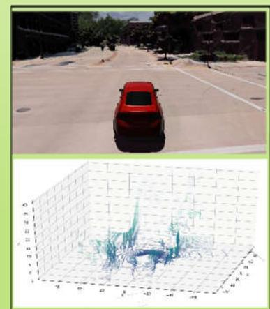
Example data from simulated camera and lidar from within a reconstructed virtual environment.
