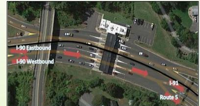
West Springfield toll plaza. An off-ramp plaza with a short distance (about 500 feet) between merging and diverging ramps, which causes a lot of weaving maneuvers and gives less longitudinal space for the drivers to switch lanes.
