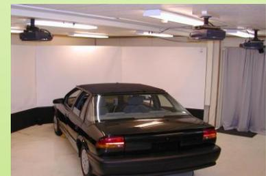
Driving simulator at Human Performance Laboratory, UMass Amherst. A full-cab fixed-base simulator with a Saturn sedan in front of three screens with three overhead projectors that provide 150 degrees of horizontal view and 30 degrees of vertical view.
