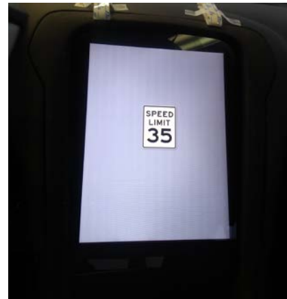
Figure 3.3 - Alert on center stack
