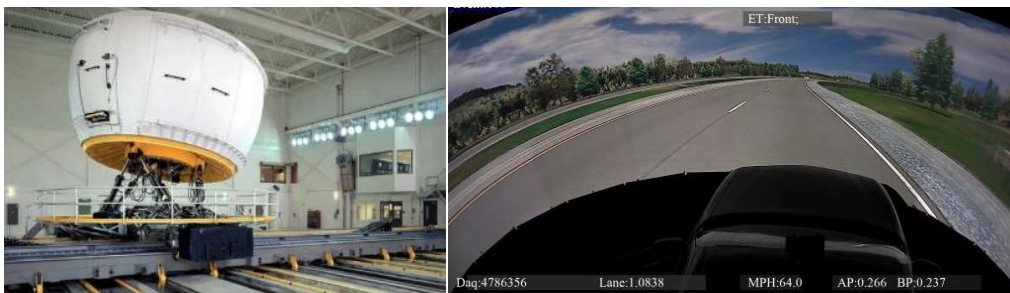
Figure 2.1 – NADS-1 driving simulator (left) with a driving scene inside the dome (right).
