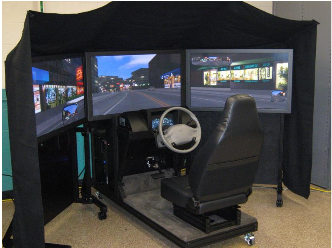
Figure 4. Quarter-cab minSim with daytime urban scene
