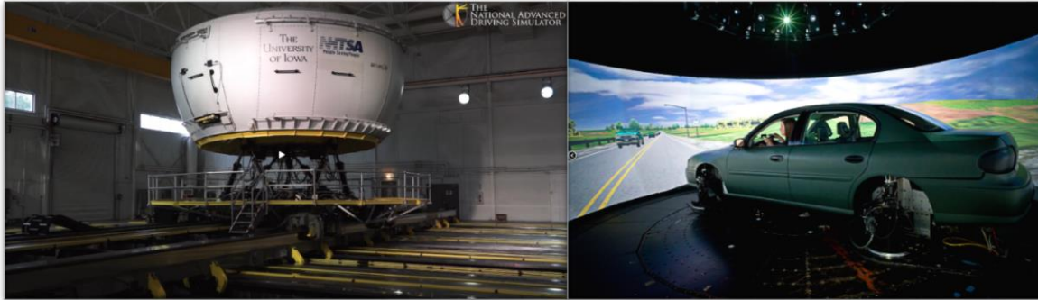
Figure 4.11 - NADS-1 high fidelity driving simulator exterior view (left) and interior dome view (right)
