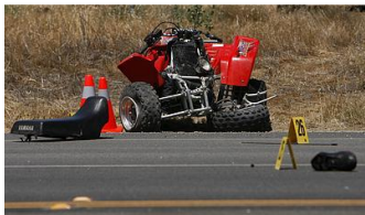
A high center of gravity, off-road vehicle tires and lack of a rear differential make ATVs and SxSs more dangerous to operate on the road than off. Roadway speeds further contribute to the risk of a crash.
