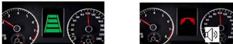
Figure 3. Automation displays activation with solid icon (left); automation requests takeover with solid icon and auditory warning (TOR) (right)
