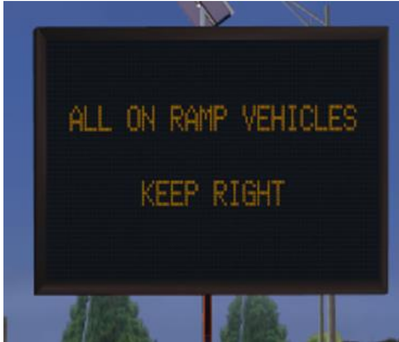
Figure 3.3 - DMS sign that will be used for the on-ramp to keep vehicles to the right
