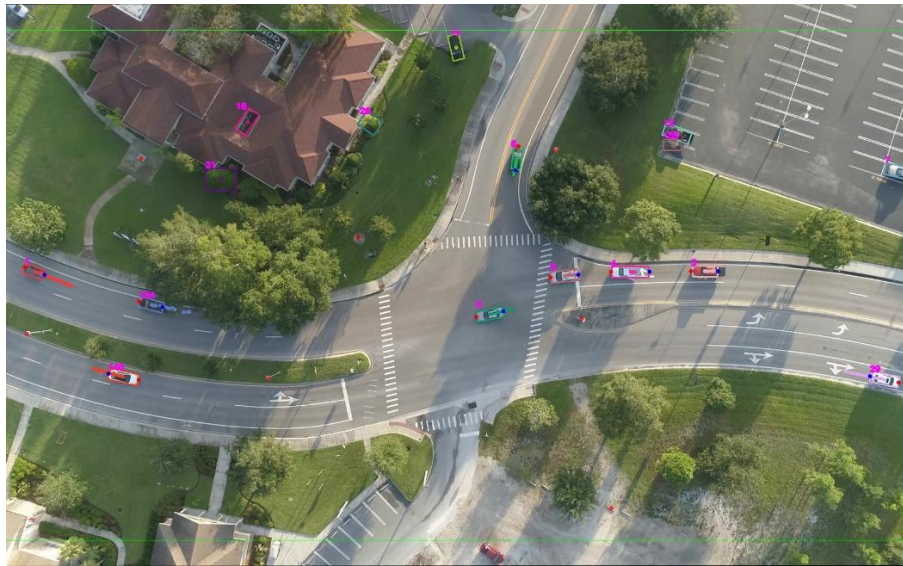
Figure 3.3 Vehicle tracking and trajectory extraction
