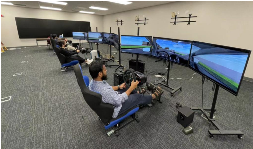
Figure 3.5 UCF SST Multi-driver driving simulator
